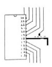
Make this cut and link arrangement to cause socket to be decoded from F800 to FFFF, so that a 2716 EPROM can be used in the standalone computer mode.
