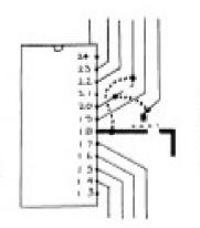
Make these cuts and links to reverse pins 18 and 20 to use NMOS BAM in this socket.
